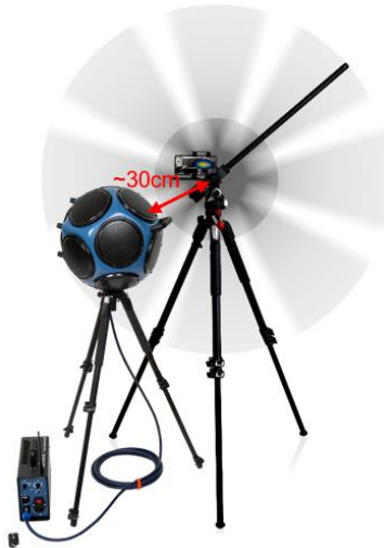
Figure 34 Sound Scanner and omnidirectional speaker located in close vicinity for conducting a reflection measurement.
