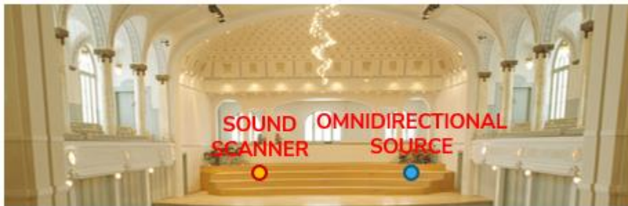
Figure 37 Sound Scanner and omnidirectional speaker located at different locations for tracking sound propagation .
