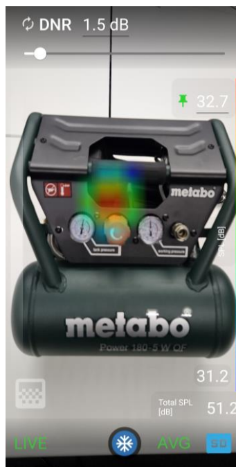
Figure 33 Press the blue indicator light to freeze and resume the LIVE stream of acoustic images.
