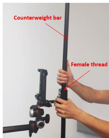
Figure 14 Tighten the connection by holding the sensor housing and turning the counterweight bar.
