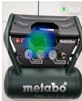
Figure 31 Press the pin icon to fix the maximum sound pressure level in the acoustic image.
