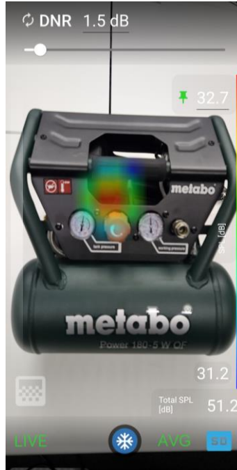
Figure 32 Press AVG for time averaging acoustic images from the LIVE stream.
